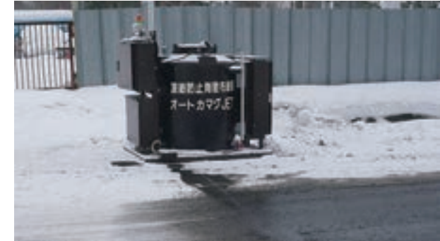
KAMAGU®, together with AUTOKAMAGU® JET, is proving highly effective against the freezing of road surfaces.
