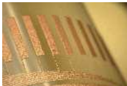
Example of use in printing of copper paste by screen printing
