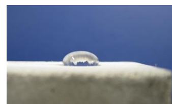
Waterproofing agent added (SYUDOX®PR-30RS)
