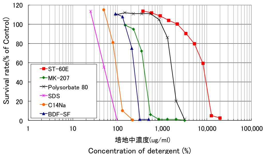
Medium: DMEM + 10%FBS, Seeding density: 20,000cells/well, Exposure time:72hrs
