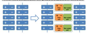
Plasticizer suppresses the approach of polymer molecules and expands between molecules
