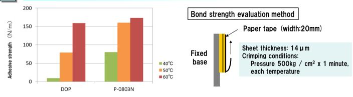
High adhesive strength can be obtained even when crimping at low temperatures.
