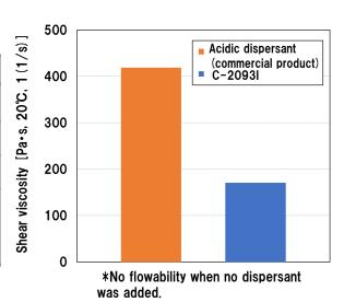
It is possible to lower the viscosity of the epoxy resin with alumina filler.
