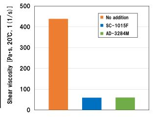
It is possible to lower the viscosity of the epoxy resin with silica filler.
