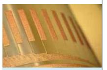
Example of use in printing of copper paste by screen printing
