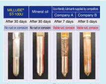
Results of anti-corrosive coatings (The shafts were soaked in a 60°C mixture of lubricant (95%) and natural seawater (5%) for a certain period of time to compare anti-corrosion performance of lubricants.)
